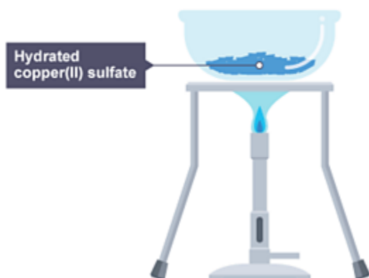
Fig. 1. A Bunsen burner is used to heat an evaporating basin containing hydrated copper(II) sulfate.
