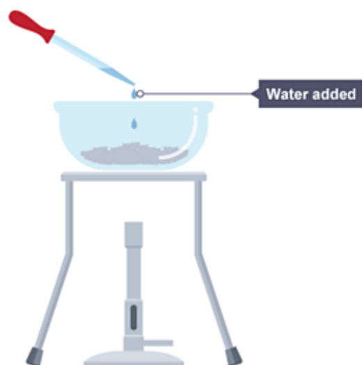
Fig. 3 The Bunsen burner is turned off and water is added using a pipette
